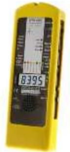
Gigahertz ME 3951A B and E Field, frequency ranges 5 to 400KHz and 2K to 400KHz
