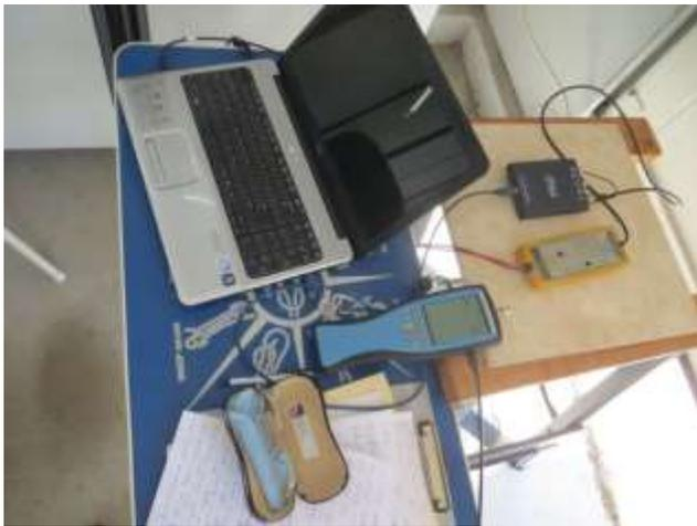
Figure 2 Laptop, picoscope and active differential probe
